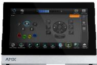
In addition, there is a smaller touch panel located on the AV cart, which allows control of the sources attached to the podium and counsel tables. This is the touch panel primarily dealt with in this manual.
