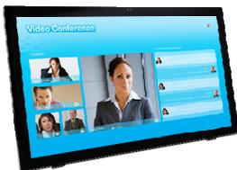
The courtrooms are equipped with three 24" touch screen LCD panels, one at the witness stand, one on the A/V cart, and one at the judge's bench. These are used for annotating the evidence being presented. At each location, witnesses, judge, or counsel can "draw" on the image being displayed on the courtroom monitors by simply touching the monitor with a finger.
